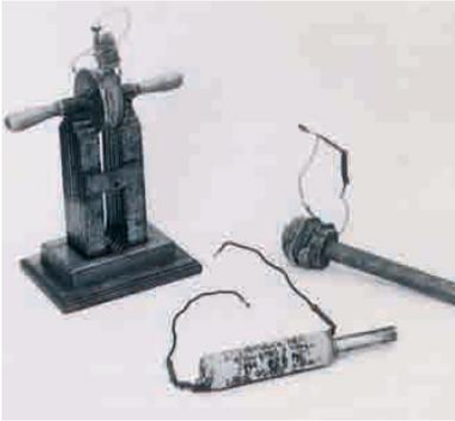
The crude inductors with which Michael Faraday discovered the law of induction.
