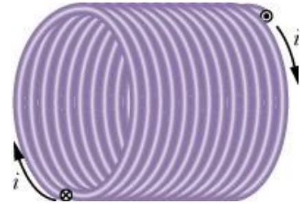
A vertical cross section through the central axis of a current-carrying solenoid
